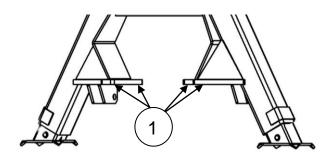
Figure 8. Connection junction on A- support legs
