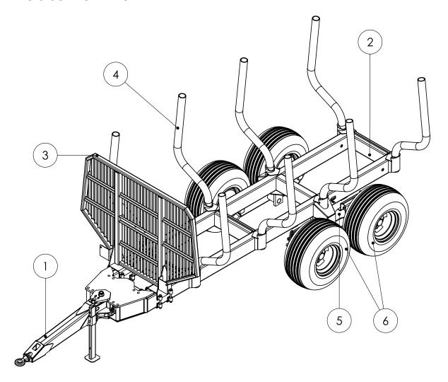
Figure 1. Basic components of Palms 10D forest trailer
