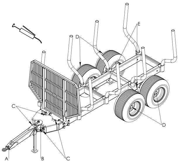
Figure 10. Lubrication points of Palms 12D forest trailer
